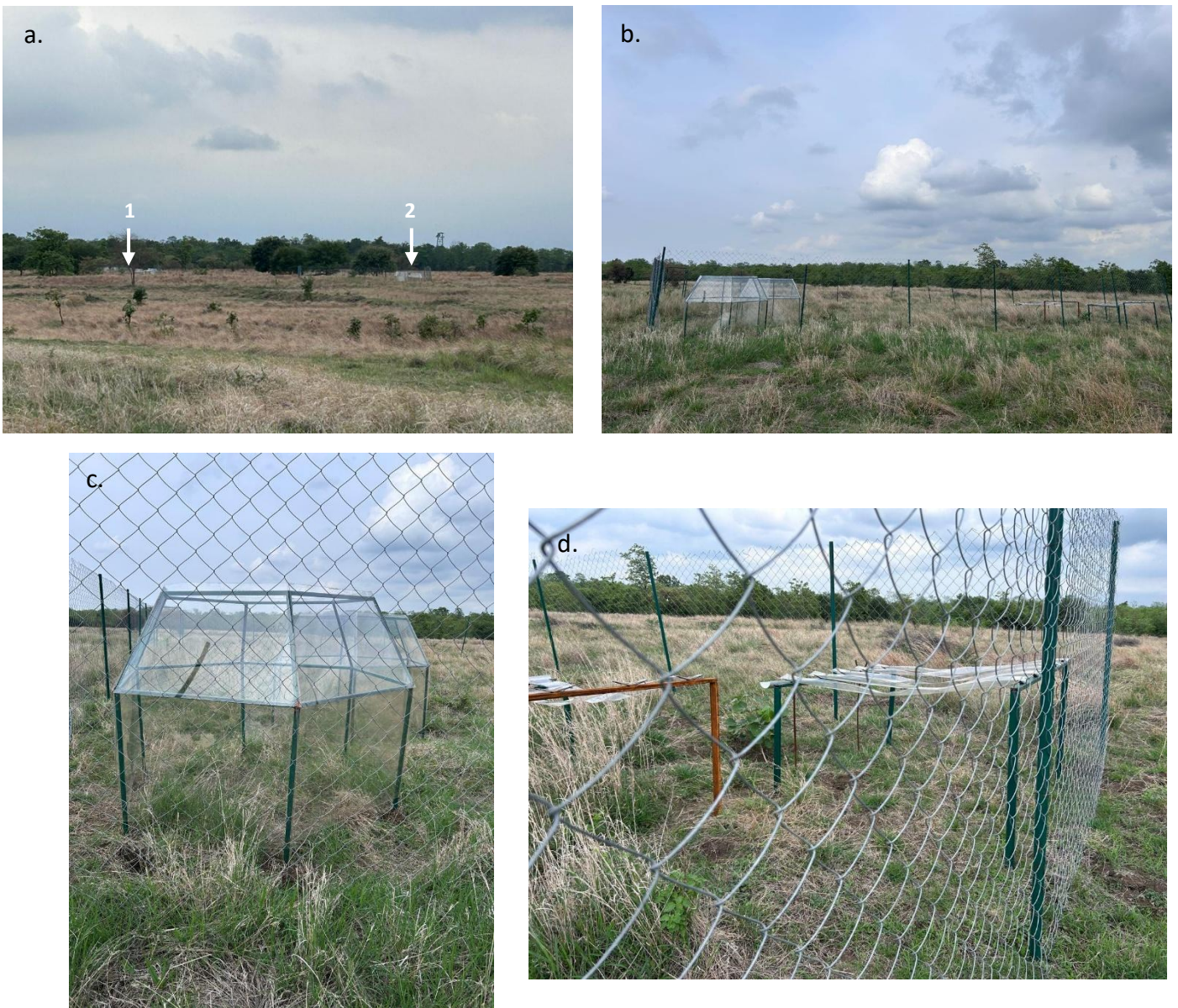
Figure 4: a. Fenced blocks 1 and 2; b. A block with Open Top Chamber (OTC) and rainout shelter; c. Close-up of an OTC installed for passive experimental warming; d. Close-up of rain-out shelter installed for imposing drought.
