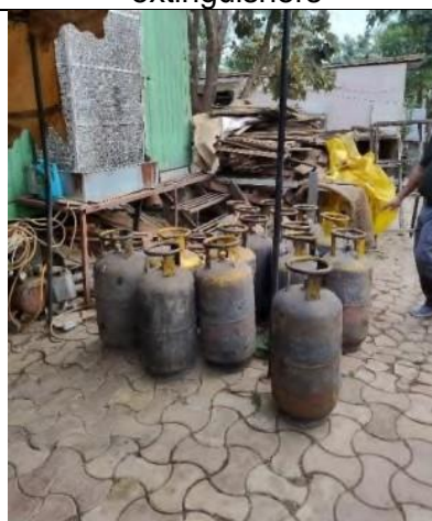
Improper storage of cylinders
