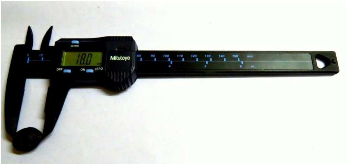
**Figure 5.2: Showing a digital vernier calipers (Mitutoyo) and how measurements are recorded**
